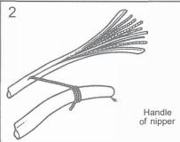
Extract the rip cord and wrap it around a suitable bar (eg handle of nippers). Pull slowly lo split the cable sheath 10the required length.
