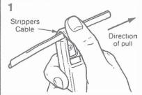
Using correctly adjusted Strippers Cable Sheath 7. make 1wodiametrically opposite longitudinal cuts on the cable sheath to expose 150-200mm of cable core.
