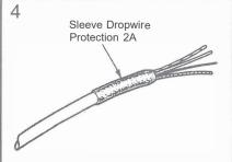
Fold back strength members along sheath and place a Sleeve Oropwire Protection 2A over the strength members and sheath.
