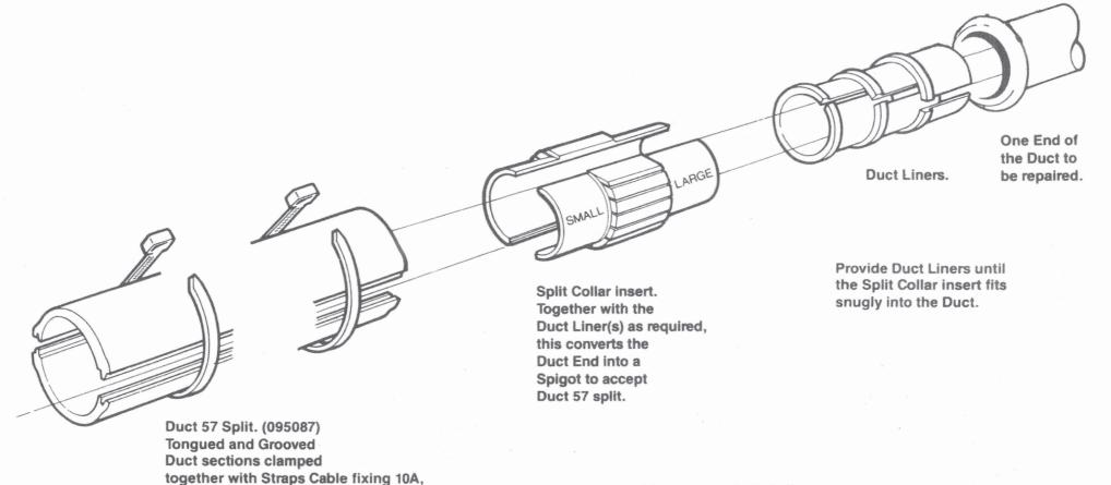
The combination of a Split Collar insert and up to three Duct Liners provides compatability for Duct Bore diameters from 98mm to 105mm inclusive in 1mm intervals. Note that the two Spigot Ends of the assembled Split Collar insert are NOT the same, being 98mm (Small) and 99mm (Large) Diameter respectively. Either Spigot will accept Duct 57 split.
