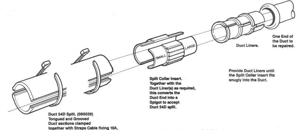
The combination of a Split Collar insert and up to three Duct Liners provides compatability for Duct Bore diameters from 88mm to 95mm inclusive in 1mm intervals. Note that the two Spigot Ends of the assembled Split Collar insert are NOT the same, being 88mm (Small) and 89mm (Large) Diameter respectively. Either Spigot will accept Duct 54D split.
