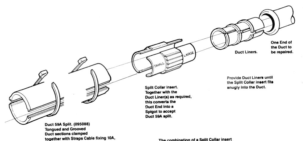
The combination of a Split Collar insert and up to three Duct Liners provides compatability for Duct Bore diameters from 73mm to 80mm inclusive in 1mm intervals. Note that the two Spigot Ends of the assembled Split Collar insert are NOT the same, being 73mm (Small) and 74mm (Large) Diameter respectively. Either Spigot will accept Duct 59A split.
